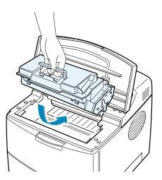
When "Ready Replace Cart" appears on the display, you need to replace the toner cartridge. Refer to the procedures under "Replacing the Toner Cartridge" on the next page.
